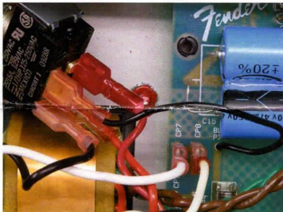
9. Move the nut on the new switch about halfway up the threads. Install the switch and use the nut and washer from the old switch to secure it. Adjust the back nut so the barrel of the switch is flush with the top of the nut. Use the provided wire ties to secure loose wires.
