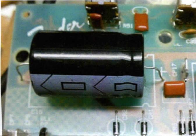
We use clear hot melt glue to secure the caps to the board and prevent vibration. You can also use a small amount of silicone sealer. Put some under the cap; you don't need much.
