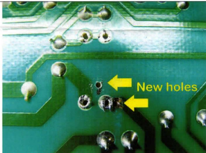
Clip the leads of R51 and R52 flush with the board. The stubs are easier to desolder and thereby prevent damage to the traces. A vacuum plunger desolderer (solder sucker) is highly recommended.
