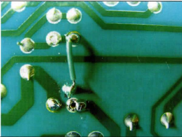
Place the trimpot through the holes from the other side. Solder one lead into the existing hole, the other into the new hole you made.
